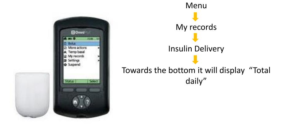
Note: You must be within 1 meter of the pod for the handset to connect
